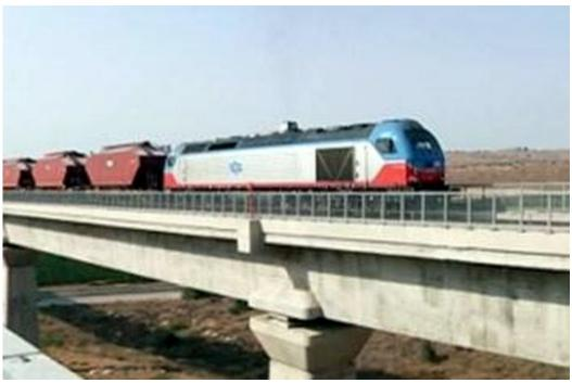
• 118:03. The first test train on the lengthy viaduct at Latrun on the new A1 line to Jerusalem. The train is loaded in order to help'settle' the trackbed and ballast. Once this line is opened next year (and electrified for operation through the tunnels) the only chance to see a Diesel locomotive or freight wagons will be when maintenance is necessary. (Image from the internet)
