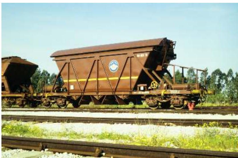
• 60-ton Coal bogie hopper no. 60001 at Kishon works, 25.2.1988 (photo: Harel Even)
