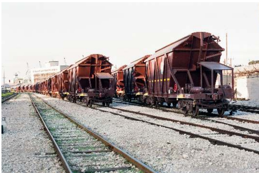
• Brand-new 60-ton coal bogie hopper wagons ex Israel Shipping Yard stabled at Haifa East Golani sidings, 2.1.1990 (photo: Harel Even)
