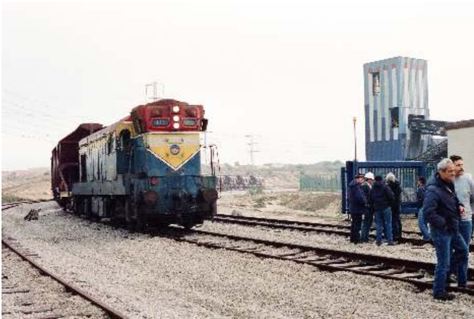
• First test train arriving at Ashdod Coal station headed by EMD G12 no. 111 with 20 empty 60-ton coal wagons, 17.1.1990
