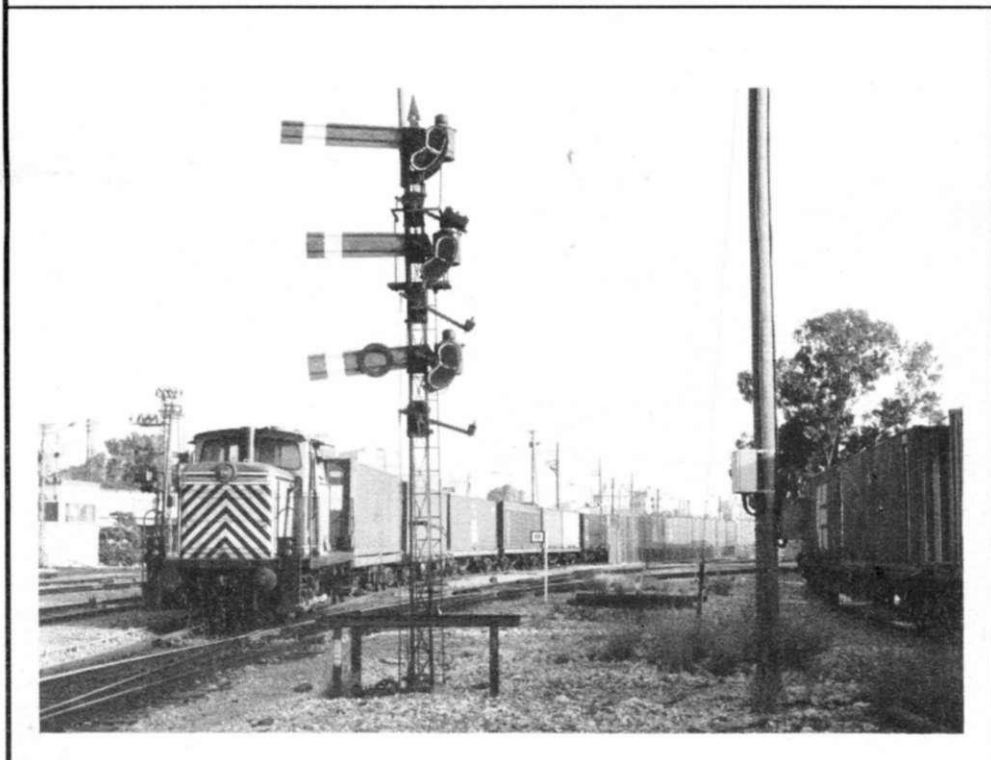
18:1 "Kilometre 0" - the datum post for all line measurements at Haifa Esat station in July 1992, as Esslingen 0-6-0D No. 221 (in new livery) hauls containers from the port past the doomed semaphores.
