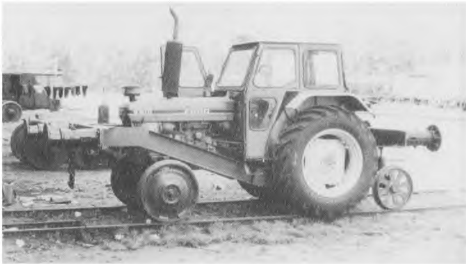
29:3: Light shunting duties at Qishon Works are carried out by this Ford tractor fitted with flanged wheels and buffing gear; seen in the north yard on 2nd. March 1989. (Paul Cotterell).
