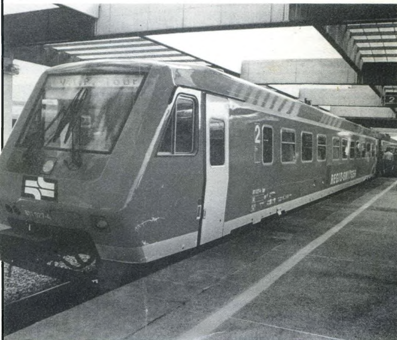
40:1: DB VT611-type 2-car tilting diesel multiple unit on trial in Israel.
