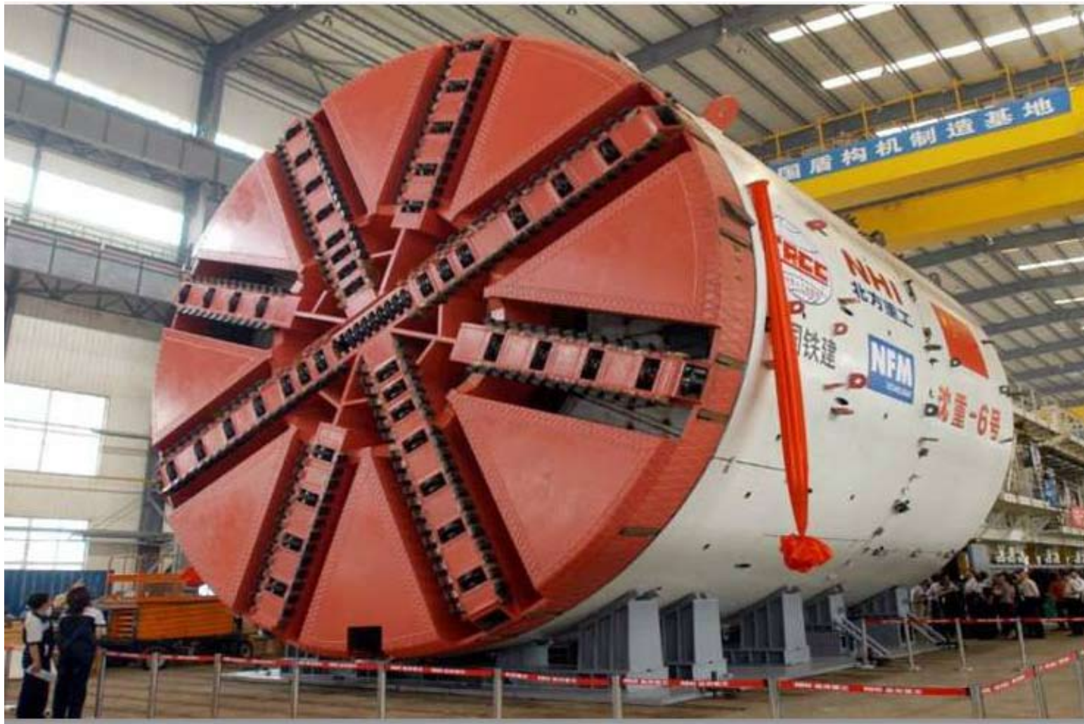
A boring picture: The Tunnel Boring Machine for the A1 Line Tunnels - Photo courtesy of Shafir Engineering.
