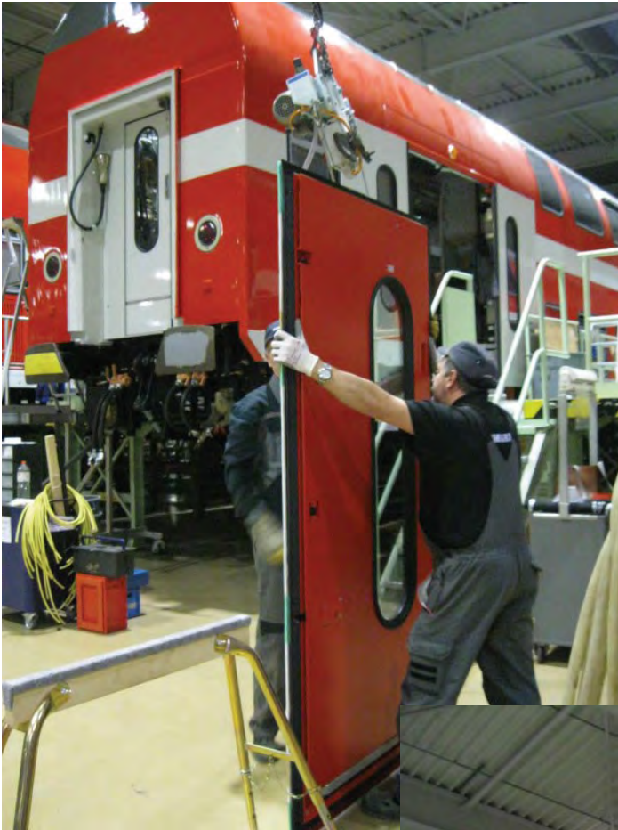
A door is ready to be attached.
