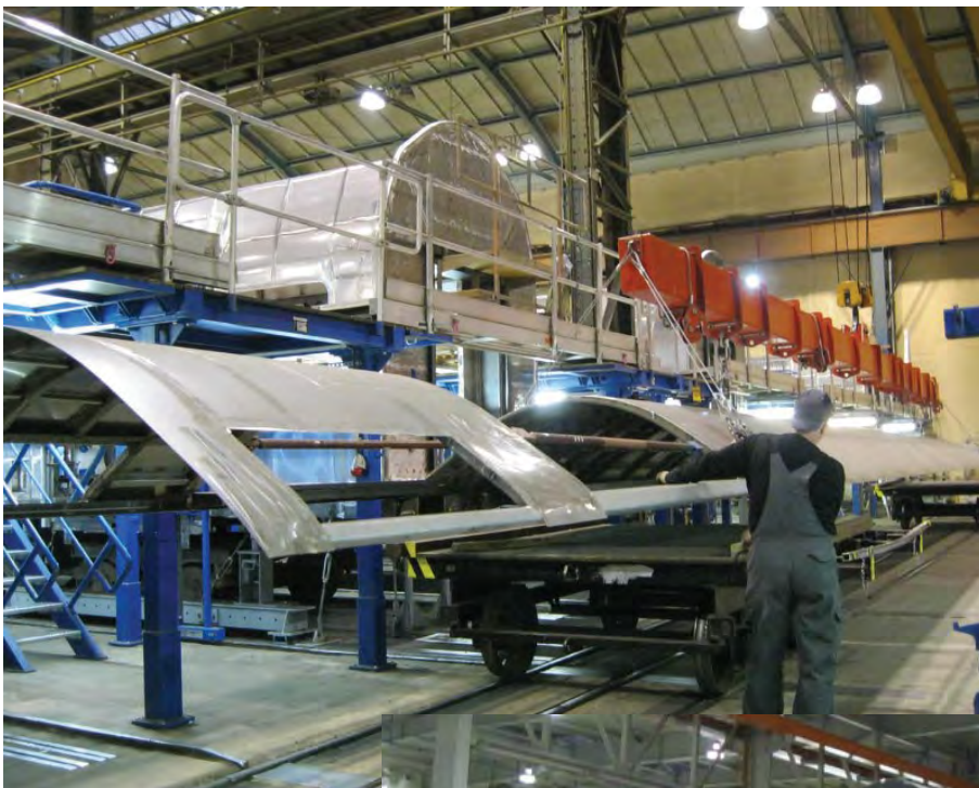
A carriage roof about to be put on.
